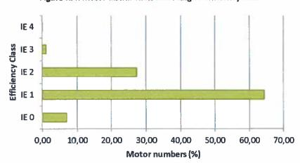
Figure K.4: Motor distribution according to efficiency class
