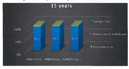
Figure M.3: A 15-year LCC analysis of an 11 kW IE2 motor<sup>60</sup>
